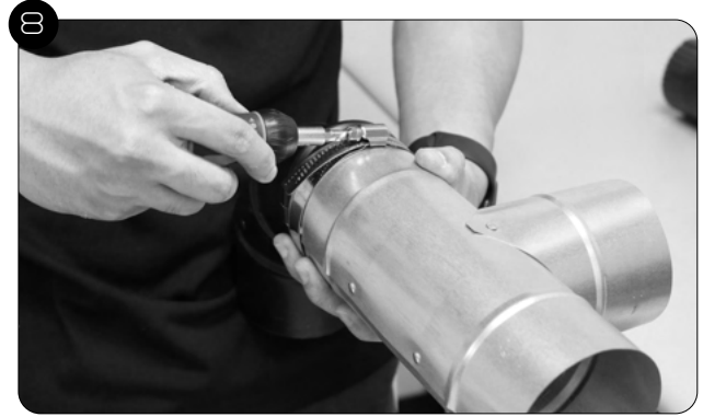
8 Secure Elbow to Ducting Tee using Hose Clamps. Repeat steps 7 - 8 with the second 3" 90° Elbow.
