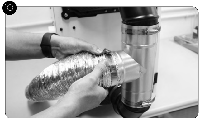
10 Attach ducting (Not Included). Exhaust accepts standard 3" ducting. Secure with Hose Clamps.
