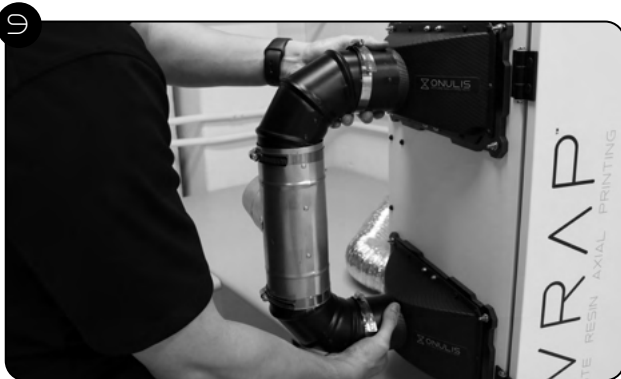
9 Attach Ducting Tees to Exhaust Plates. Secure with Hose Clamps.
