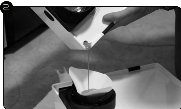
Pour resin from the old Vat into the new Vat, using a Disposable Filler Filter.
