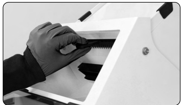
Push Vat Cleaning Tool into holes above Drip Comb, using a downward U-shape motion. Move Cleaning Tool back and forth, letting any resin drip into Resin Catch.
