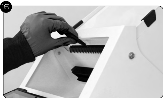
Push Vat Cleaning Tool into holes above Drip Comb, using a downward U-shape motion. Move Cleaning Tool back and forth, letting any resin drip into Resin Catch.
