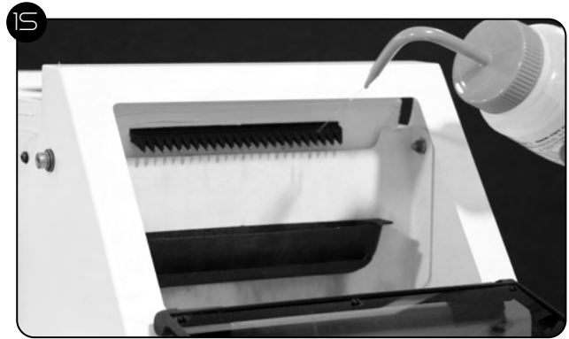
Very Important: To avoid clogging, spray isopropyl alcohol on Drip Comb face. Allow to drain in Resin Catch.
