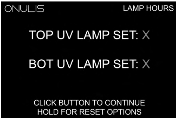
UV Lamp run-time listed for top and bottom light array. Click button to continue. Hold button to reset.
