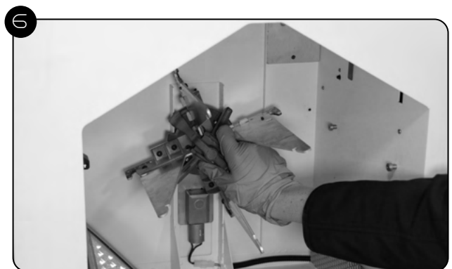
Push Mandrel Carriage Latch onto drive shaft, rotate clockwise until click.
