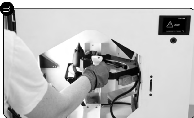
Open door. Place DLP parts on Curing Table. If parts are longer than 9.5 inches, use optional Static Curing Table.* Close door.
