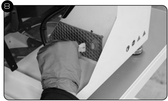
Connect plug on Curing Table cord to socket located in lower right corner of mounting wall.
