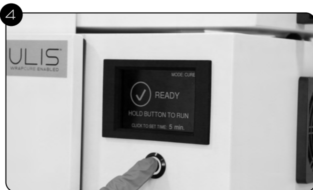
Push button to set curing time. Curing time options: 5 – 30 minutes, in 5 minute increments.
