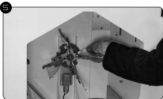
Insert Mandrel Carriage, installing on back machine post. Align spokes with slots in rear mount plate.
