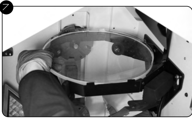
Place Curing Table on Curing Table Frame.
