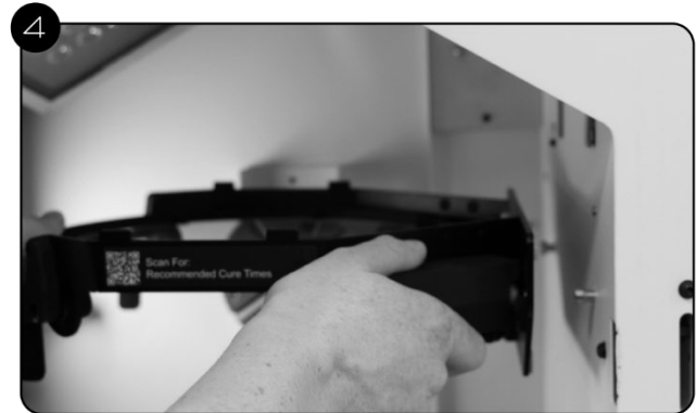
Hold sides of Curing Table Frame, lifting off Mounting Posts and remove from machine. Set aside.
