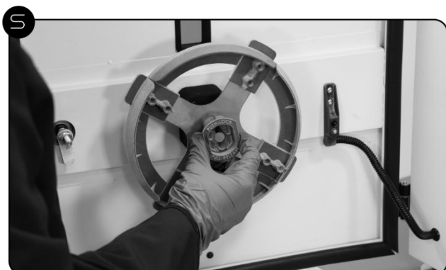
Pull Latch to release Rotating Guide and remove it from door.
