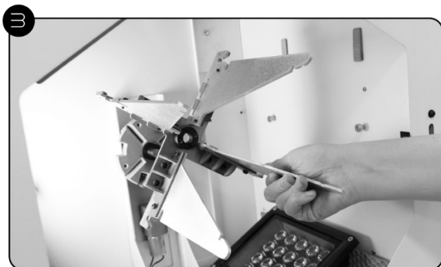
Hold spokes of Mandrel Carriage, pulling forward to remove from machine. Set aside.
