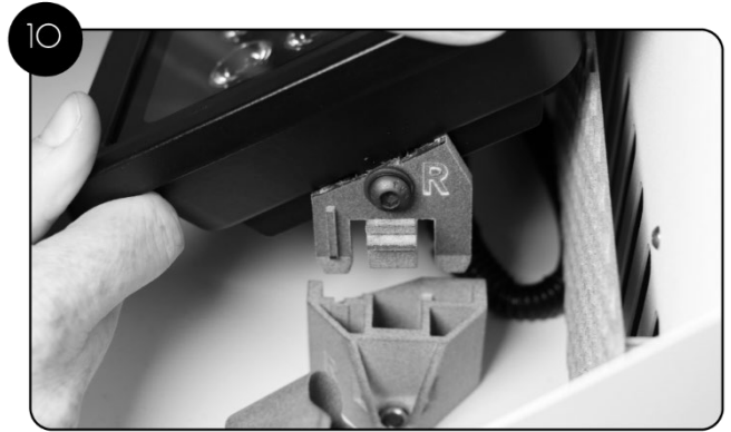
Insert plug on front of light into corresponding socket in front of machine.
