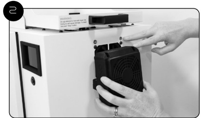
Line the screws in the Driver Pack up with the mount holes on the machine.
