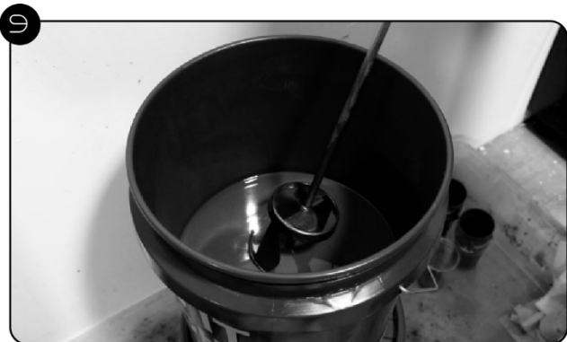
Recommended: To ensure a consistent print, mix your resin prior to filling the Vat. When waste resin sits, mineral oil rises to the surface of the mixture. Stirring the resin prevents an excess of mineral oil in each print.
