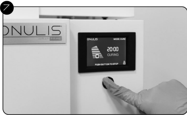
Depress and hold button to start curing cycle.
