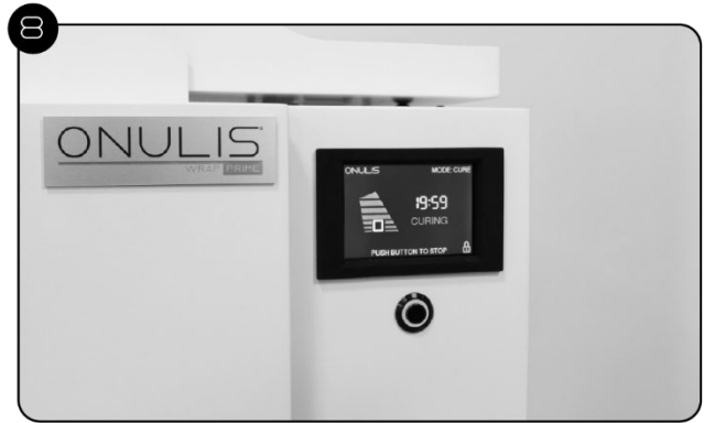
Curing will stop: a. When timer ends, or b. When button is pressed.
