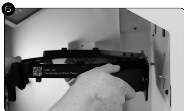
Install Curing Table, aligning mounting holds on side of Curing Table Frame with Mounting Posts on right side of lower machine chamber.
